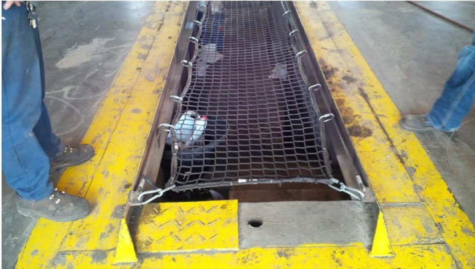
Here's a solution for preventing falls into oil change pits from our friends at Louisiana Scrap, Port Allen, Louisiana. The carabineers at the end detach and the entire netting pushes easily to the center of the pit for full access to the underside of the equipment. In the photo below, notice the solid platform built across the center of the pit to allow forklifts to pull onto the pit sideways, allowing the mechanic to service a forklift from below.
