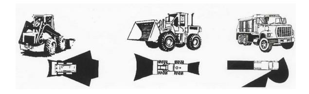
A "blind spot" is any area that a driver can't see by looking around or by using his or her mirrors, and they can be a big problem in the recycling processing operations. Blind spots are caused by the way the equipment has been designed to get the work done. In the example, the shadowed areas around each piece of equipment represent a blind spot. If someone or something is in this area, it will be invisible to the driver or operator.
