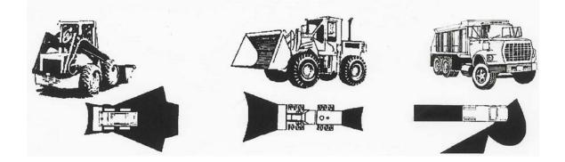
A "blind spot" is any area that a driver can't see by looking around or by using his or her mirrors, and they can be a big problem in the recycling processing operations. Blind spots are caused by the way the equipment has been designed to get the work done. In the example, the shadowed areas around each piece of equipment represent a blind spot. If someone or something is in this area, it will be invisible to the driver or operator.
