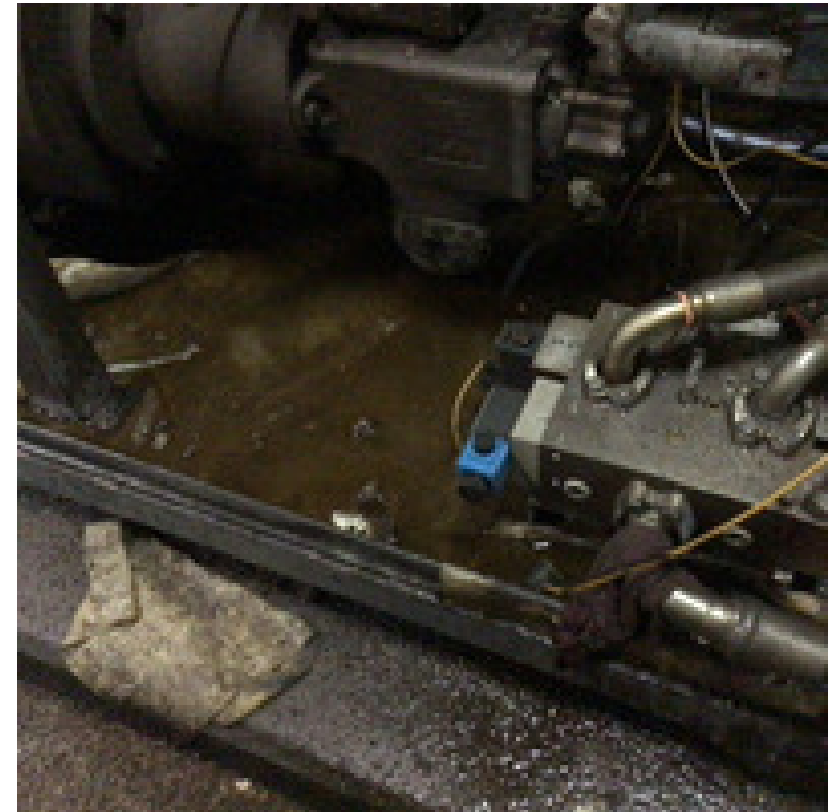
Oil and grease build-up
