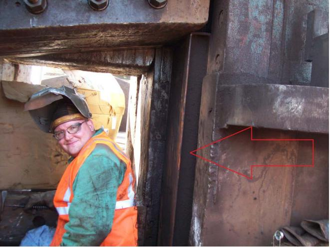
As part of your Lockout procedure, make sure you eliminate the danger presented by gravity when working inside a machine. In this shear for example, this welder is using an I-beam as a block. He's welded solid ends on the I-beam to help keep it in place and make it more substantial. This is a great idea especially with older equipment that does not have a mechanism to pin up the head.
