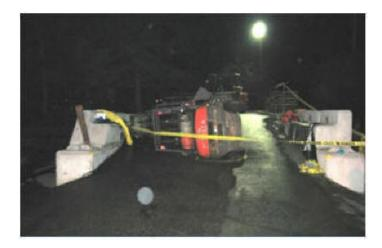
This photo shows that scene of a fatality that occurred when a forklift tipped over and the operator thought he could "jump clear." He didn't quite make it. He was crushed between the forklift rollover bar and the concrete floor. He wasn't wearing his seatbelt.
