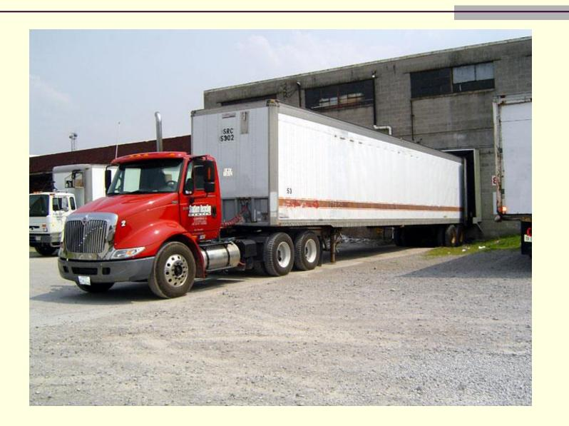
A 47-year-old man was operating a forklift in the bed of a semi-trailer. As the truck driver was pulling away from the dock, the forklift fell from the trailer bed to the ground...The lift operator was able to get himself off the ground and enter the facility, where he was treated by medical personnel. Approximately 16 hours later he died as a result of the injuries he suffered.
